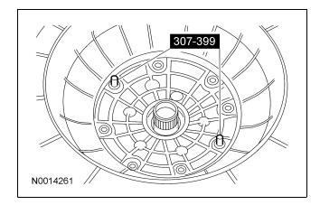
82. CAUTION: The special tools must be used to correctly align the pump with the adapter plate to reduce gear noise, bushing failure and leakage.
